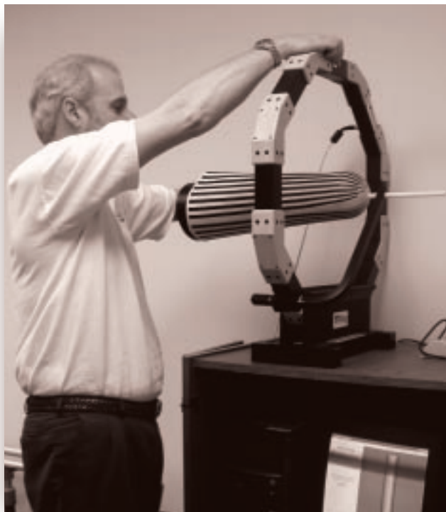
Gus Eppinger uses a T-ring, which digitally records shape measurements used to fabricate a socket for a new limb.
